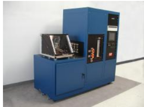
Refrigeration Compressor Test Stand – controlled by quad PID loops in Aromat PLC, includes data acquisition and HMI
