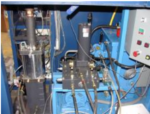
TetraTek Products, Inc. - Servo- Hydraulic Pulse Generator controlled by Allen Bradley PLC
